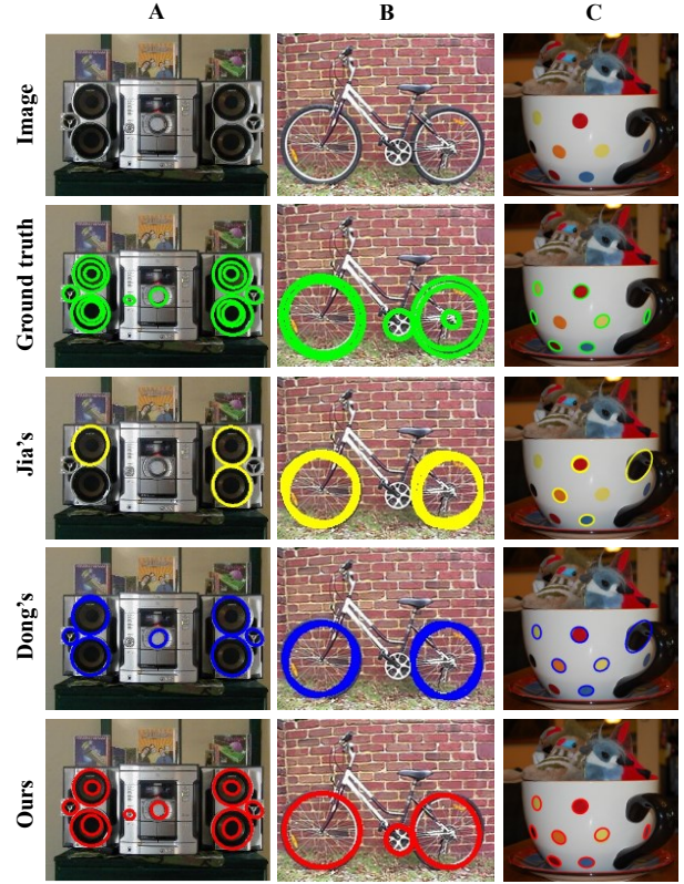
Figure. 6. Examples of ellipse detection in the combined public dataset. Green ellipses indicate ground truth. Dong's detector results are represented by blue ellipses. The detected results based on the proposed detector are visualized by red ellipses.
