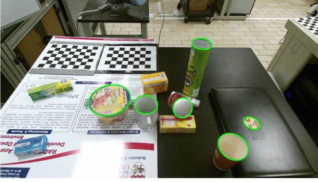
Fig. 15. Real-time ellipse detection in a sequence of 214 images. A cluttered background with light and dark colors is used to verify the robustness of the presented detector.
